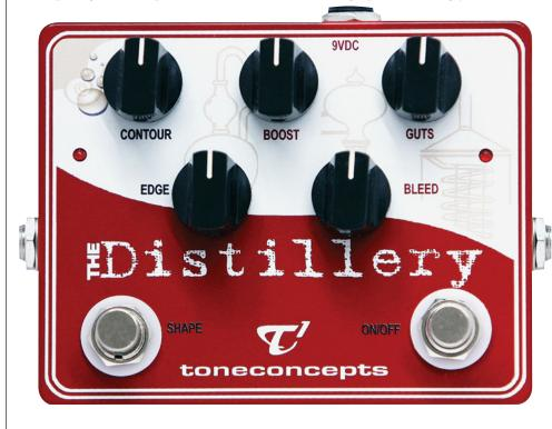
bypass pedal, it features two circuits, each activated by a footswitch. The right footswitch is the On/Off button for a boost circuit featuring three controls: The Boost knob gives 20 dBs of added volume and edgy grit; the Guts knob is an extra gain stage to add more punch and sustain; and the Bleed knob is a passive tone shaper that can tame highs or add edge. These features would be more than enough for the guitar-
